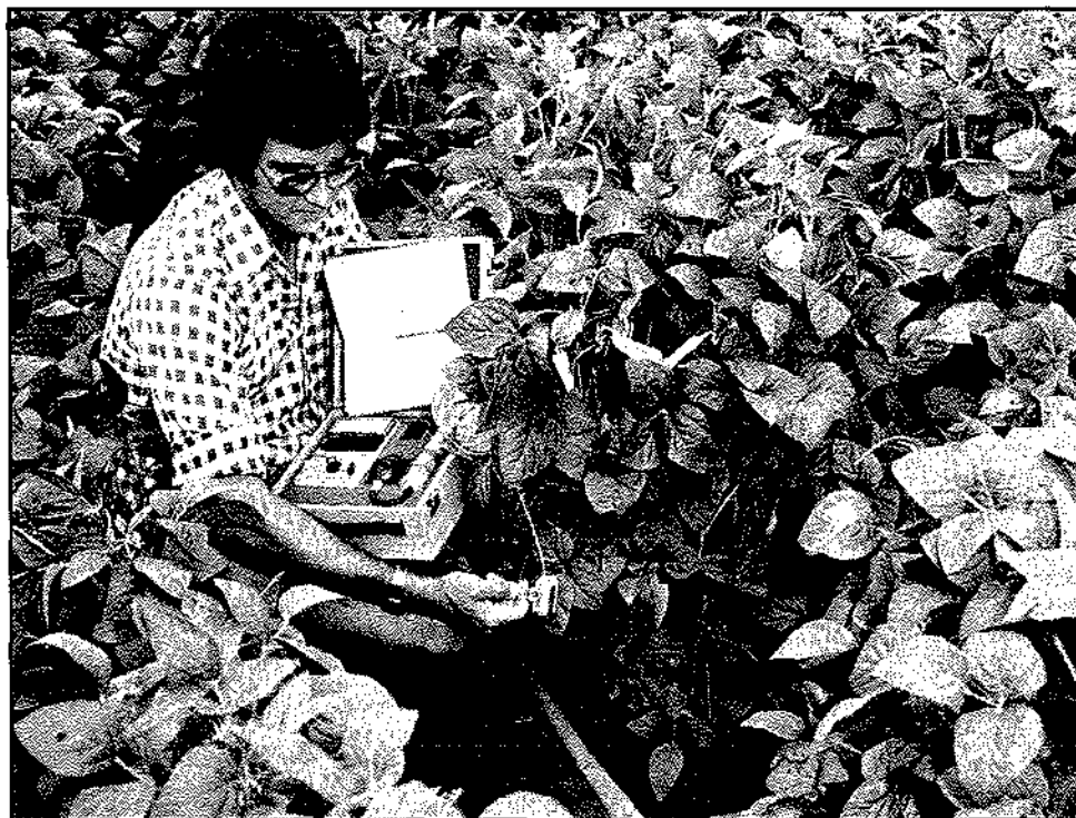
A diffusion porometer is used to measure the rate with which water vapour moves through the stomata of a leaf and this indirectly indicates the internal moisture status of the plant
