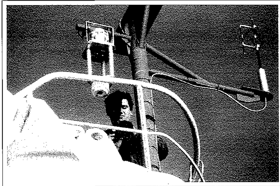
Highly sophisticated instrumentation being installed on the research vessel SA Agulhas by Dr Mathieu Rouault of the University of Cape Town in order to study the effect of the ocean on the overlying atmosphere and ultimately on Southern Africa's weather. (Photo: Prof JRE Lutjeharms, University of Cape Town)
